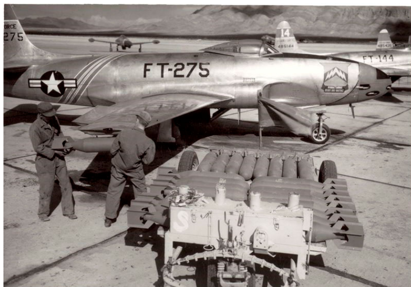
A 56th Fighter Wing Lockheed F-80 Shooting Star being loaded with munitions in 1949.
